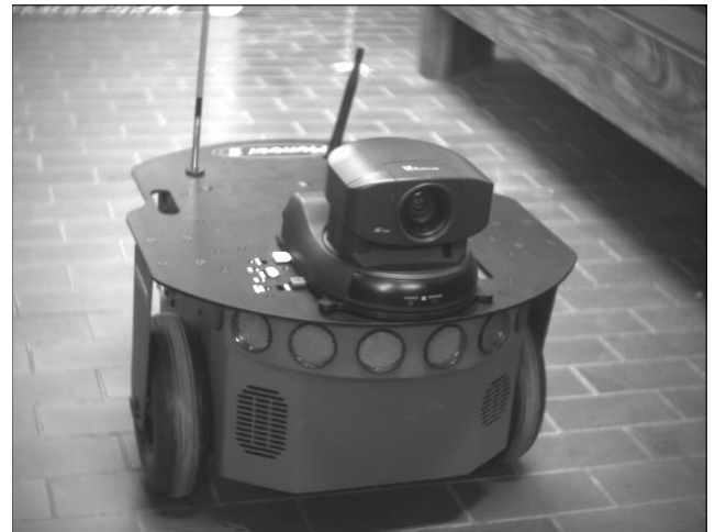
Figure 2: The mobile robot Pioneer 2 DX.
