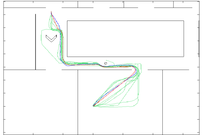
Fig. 4. Step #1 of the first task: trajectory followed by the Tangential Escape architecture (red), trajectory followed by the specialist (blue) and similar trajectories followed by the volunteers (green).
