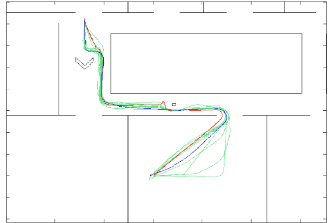
Fig. 5. Step #2 of the first task: trajectory followed by the Tangential Escape architecture (red), trajectory followed by the specialist (blue) and similar trajectories followed by the volunteers (green).
