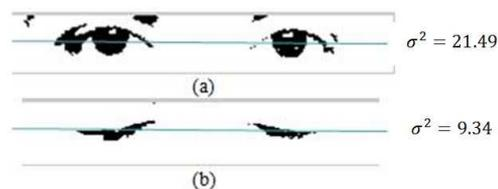
Figure 6: Dispersion of eyes pixels around the average for the eyes opened (a) and eyes closed (b).
