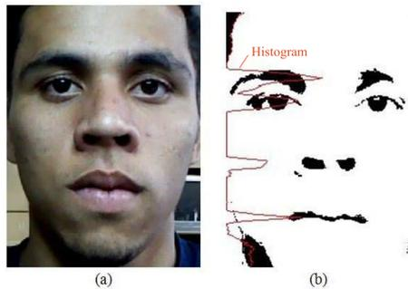
Figure 4: (a) Photo of an user face and (b) horizontal histogram in binarized image.
