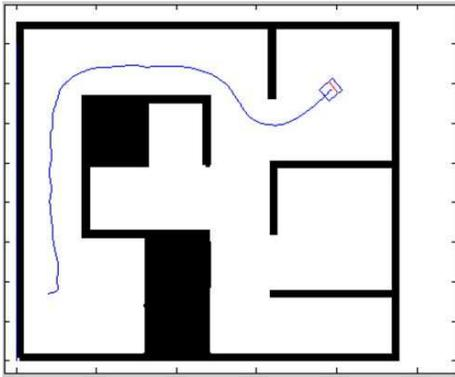
Figure 11: Trajectory executed by the robot from living room to bedroom 1.
