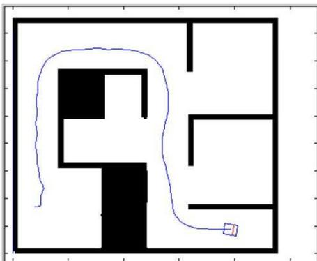
Figure 13: Trajectory executed by the robot from living room to service area.
